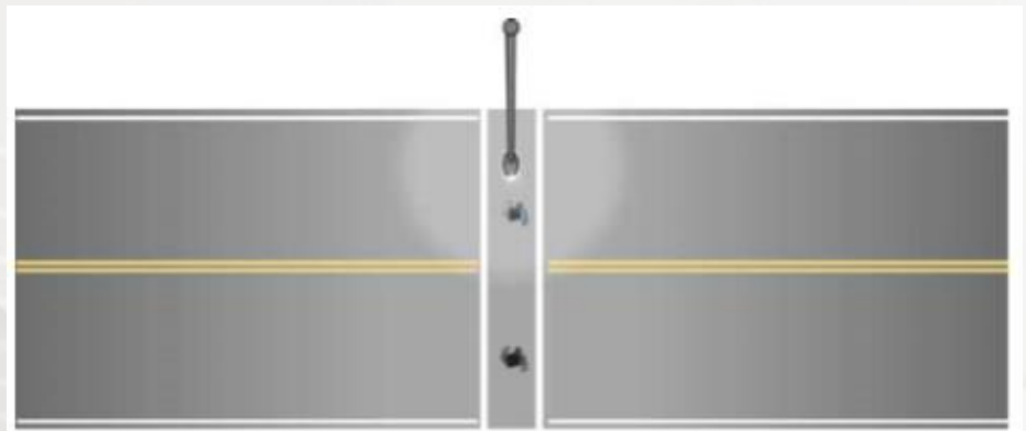
Figure 11. Drawing. Traditional midblock crosswalk lighting layout.
