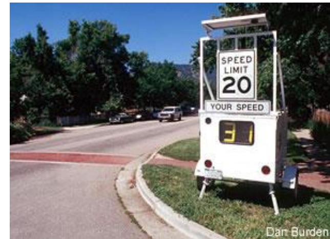
Figure 24 - A speed limit trailer communicates driver's speeds as they drive by.
