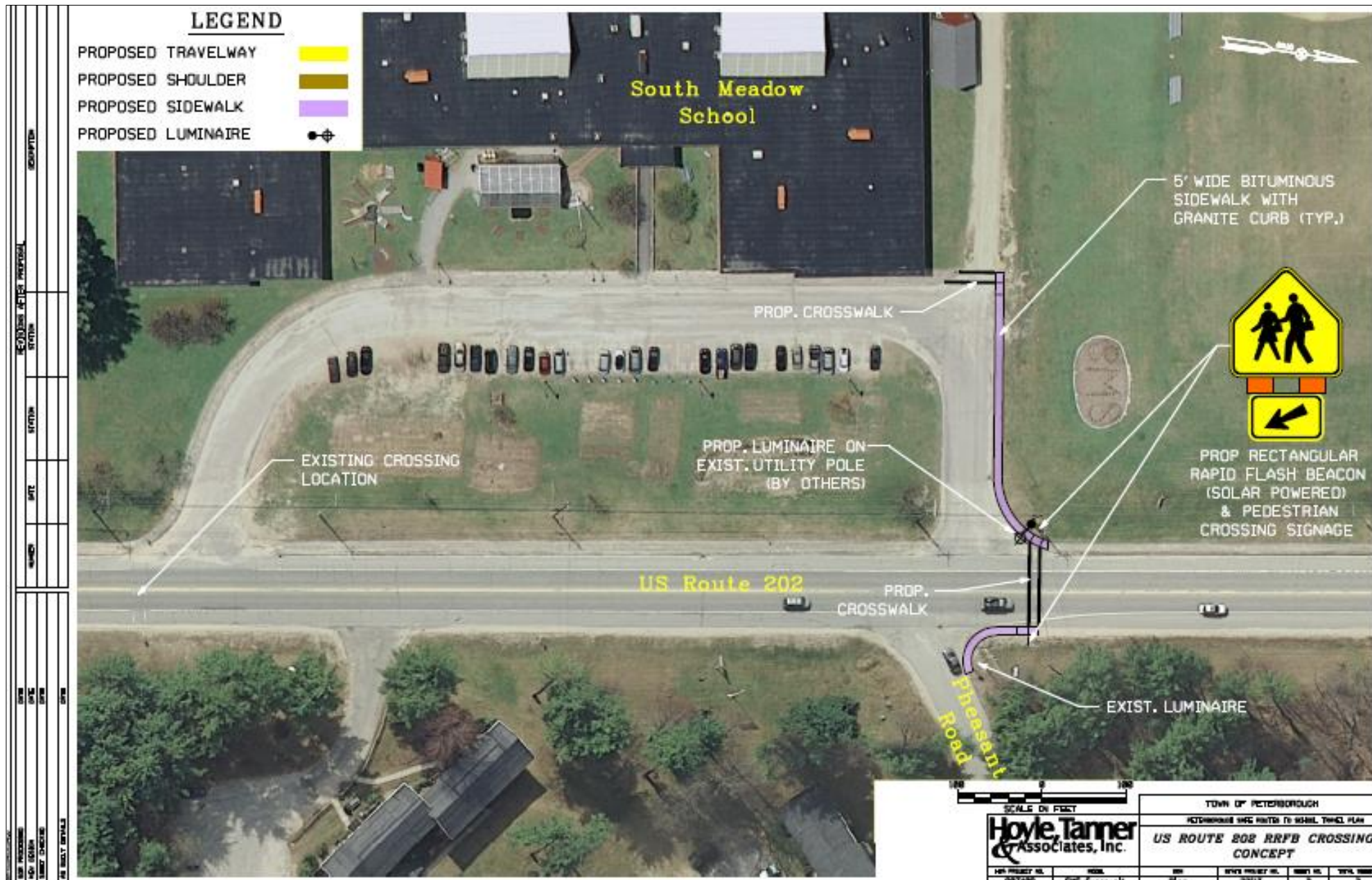
Figure 12. Proposed Safety Improvements to the Crossing on U.S. Route 202 to SMS
