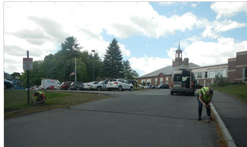
SWRPC staff installing a traffic counter at Site 3 in the school entrance.
